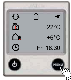
Control panel in standby
